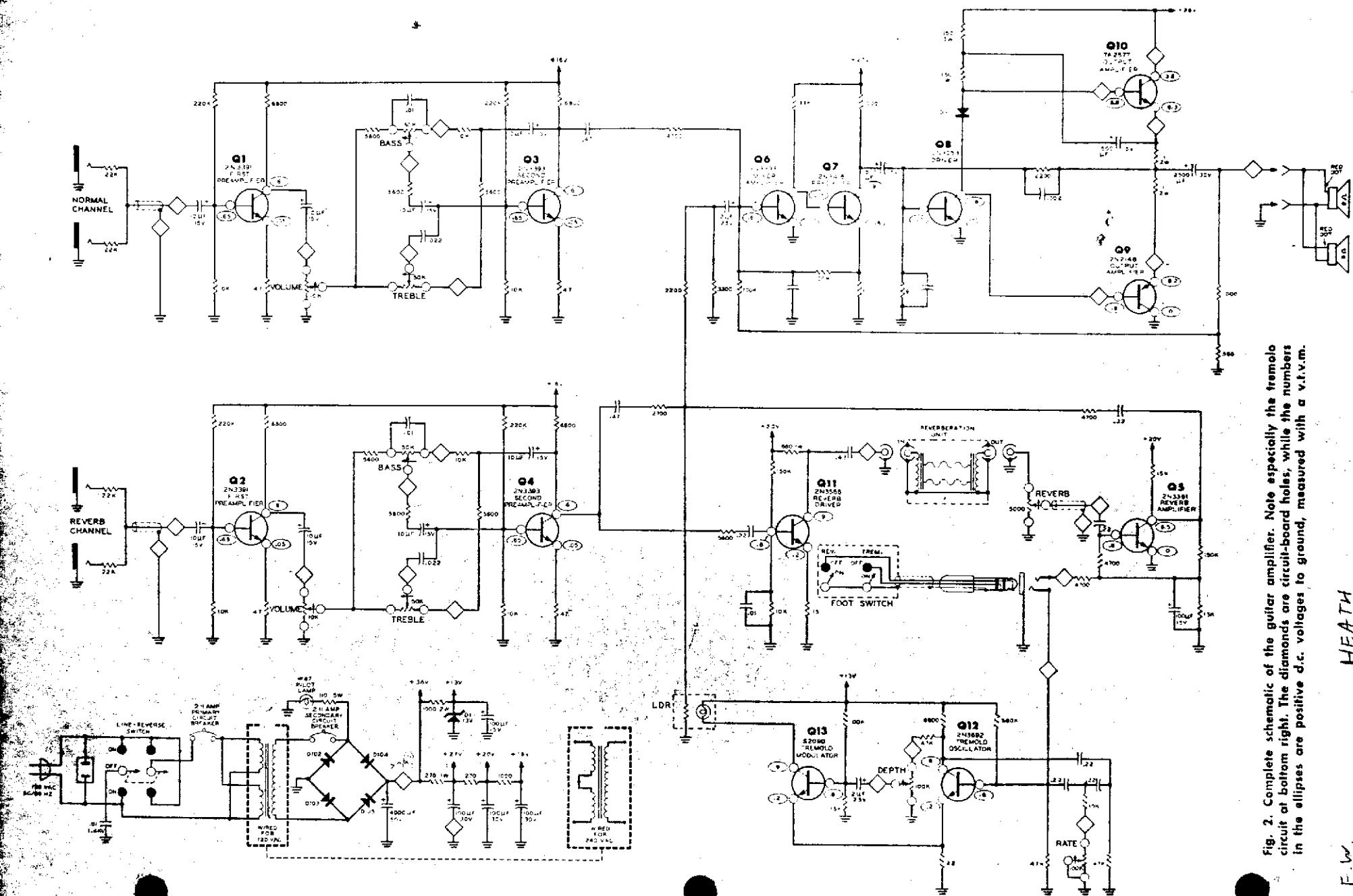
Fig. 2. Complete schematic of the guitar amplifier. Note especially the tremolo circuit at bottom right. The diamonds are circuit-board holes; while the numbers in the ellipses are positive d.c. voltages measured with a v.t.v.m.
